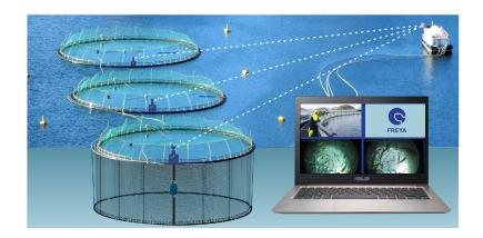
**In the Fisheye software** you can open all cameras, control light, read sensor values and control the winch. **For navigation:** Highlight camera window and use arrowkeys or controller in software. The software alerts the user by changing color from green to red on the component in the system chain that is malfunctioning. There is also a overview to identify where the fault lies in the system. This makes troubleshooting very efficient.
