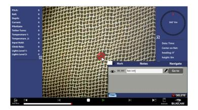
During inspection, data is retrieved from ROV together with time stamp, depth, direction, speed, temperature and more.
